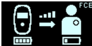
Figure 47: FCE Charging IPG Status Screen
