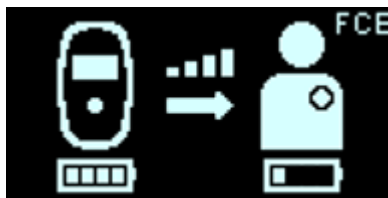
Figure 62: FCE Charging IPG Status Screen
