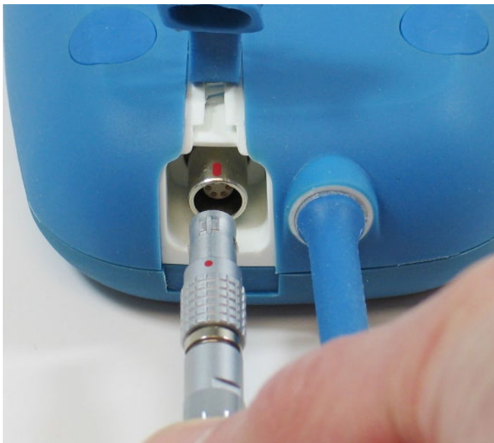
Figure 8: Alignment of the DC Connectors
