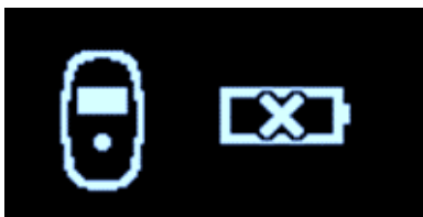
Figure 21: Low Charger Battery Alert Screen
