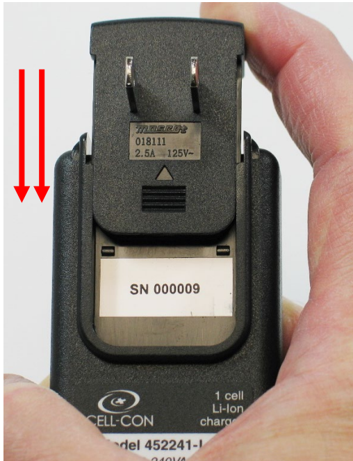
Figure 6: Installing the Plug Adapter
