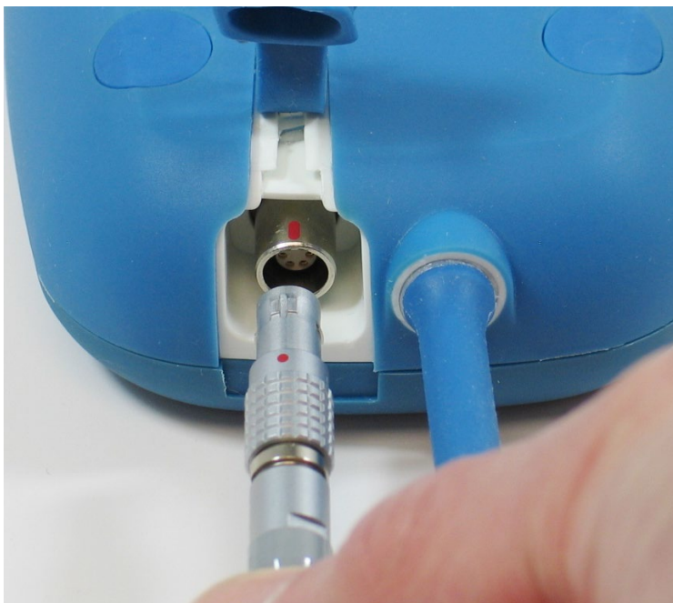
Figure 8: Alignment of the DC Connectors
