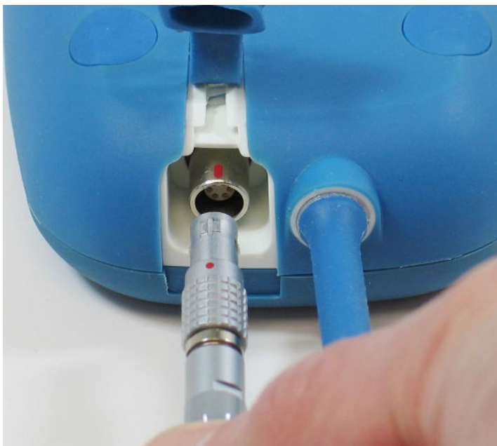
Figure 8: Alignment of the DC Connectors
