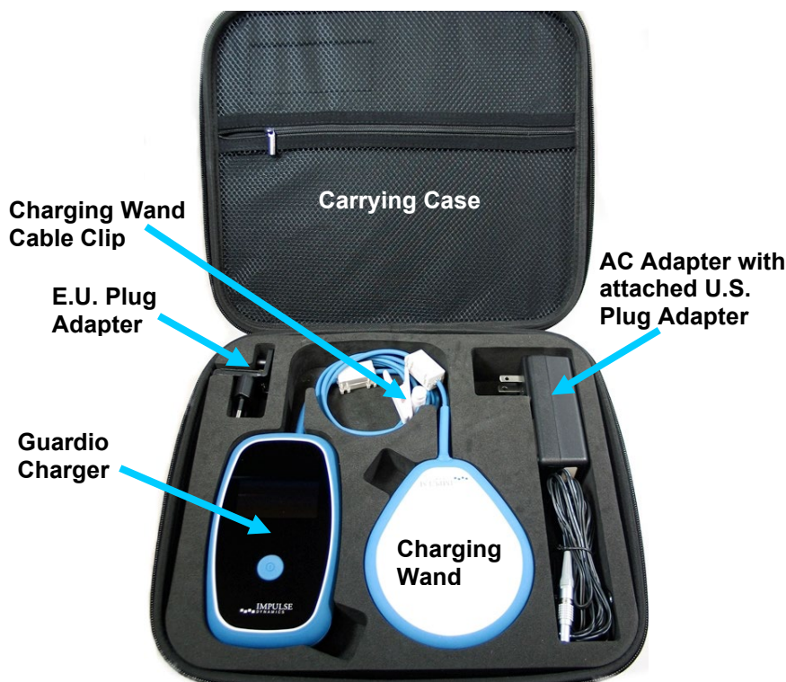
Figure 1: Guardio Charger System Components
