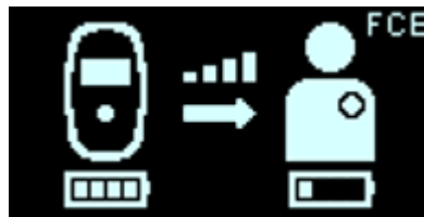
Figure 52: FCE Charging IPG Status Screen
