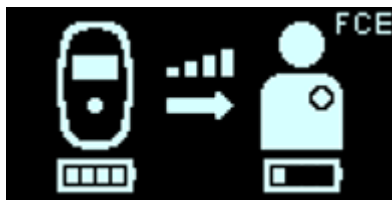
Figure 97: FCE Charging IPG Status Screen
