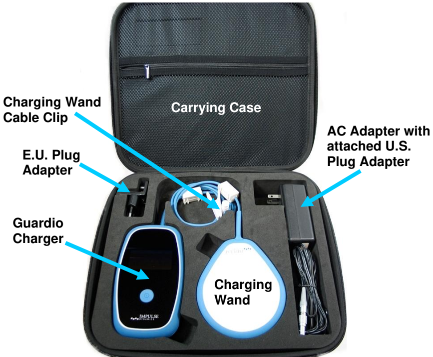
Figure 3: Guardio Charger System Components
