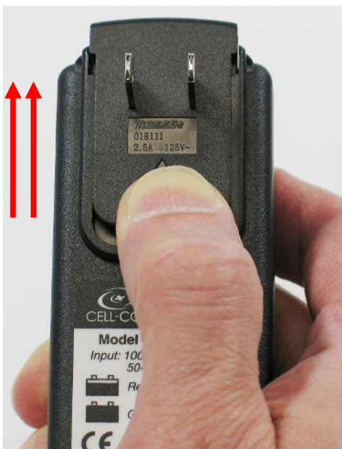
Figure 5: Removing the Plug Adapter
