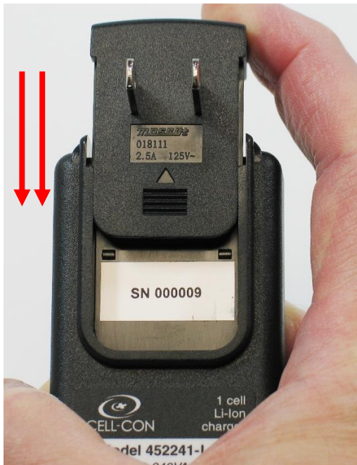
Figure 6: Installing the Plug Adapter
