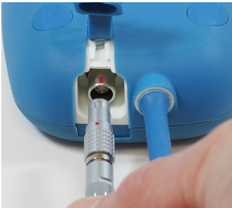
Figure 8: Alignment of the DC Connectors
