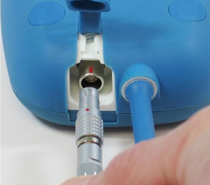
Figure 3: Alignment of the DC Connectors
