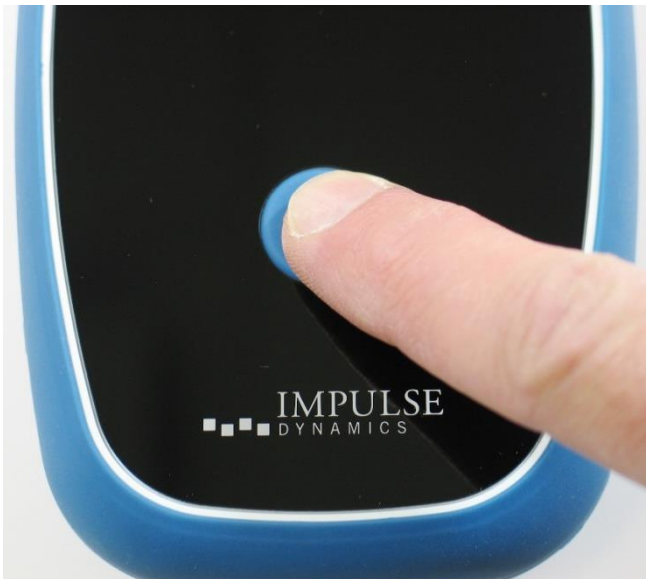
Figure 6: Pressing the Power Button on the Charger
