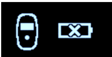
Figure 21: Low Charger Battery Alert Screen
