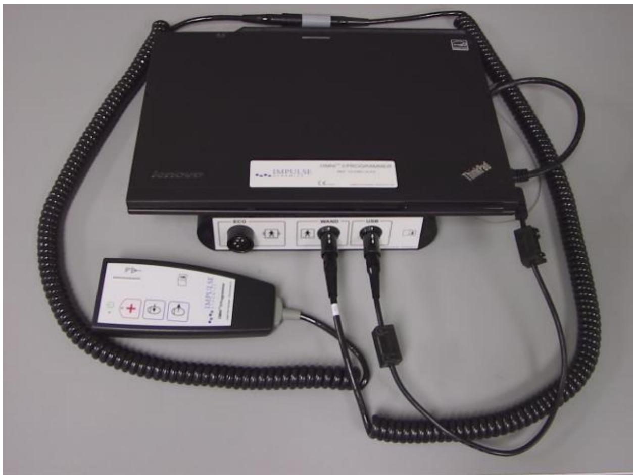
**Figura 1: L-OMNI II Programmer (bl-OMNI Smart Software) u l-Programmer Wand**
